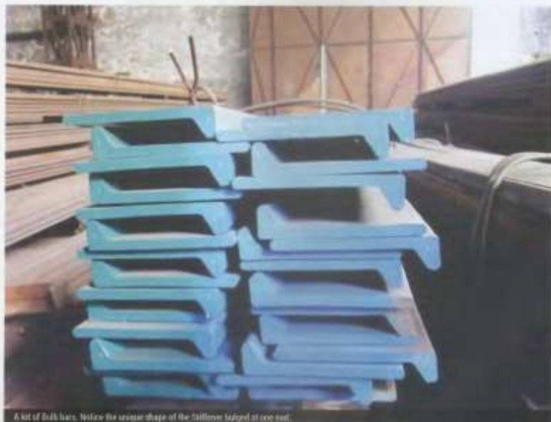
A lot of Bulb bars. Notice the unique shape of the 500mm legged at 100 mm.
